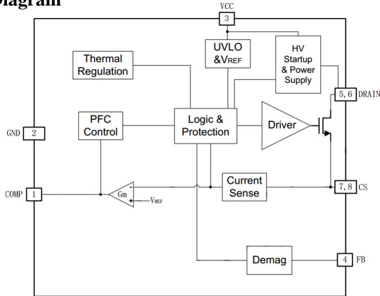
Figure 3. JH5442TL7 Internal Block Diagram
