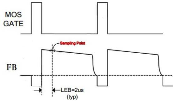
Figure5.Feedback voltage detection
