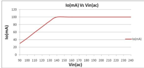
Figure4. Io - Vin relation curve
