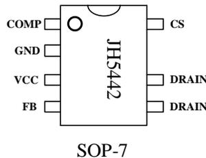
Figure 2. Pin Configuration
