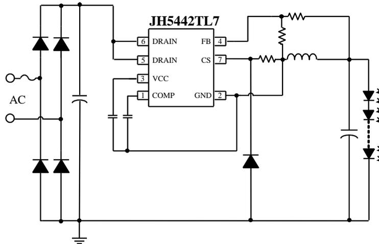
Figure 1. Typical application circuit for JH5442TL7
