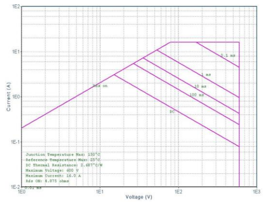
Maximum Safe Operating Area For JCS5N60FC
