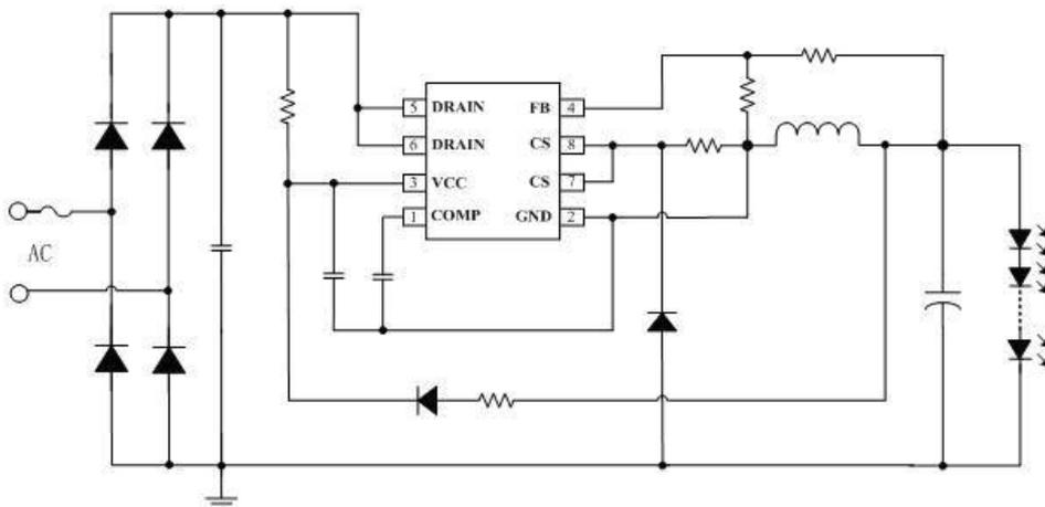
Figure 1. Typical application circuit for HW9616B
