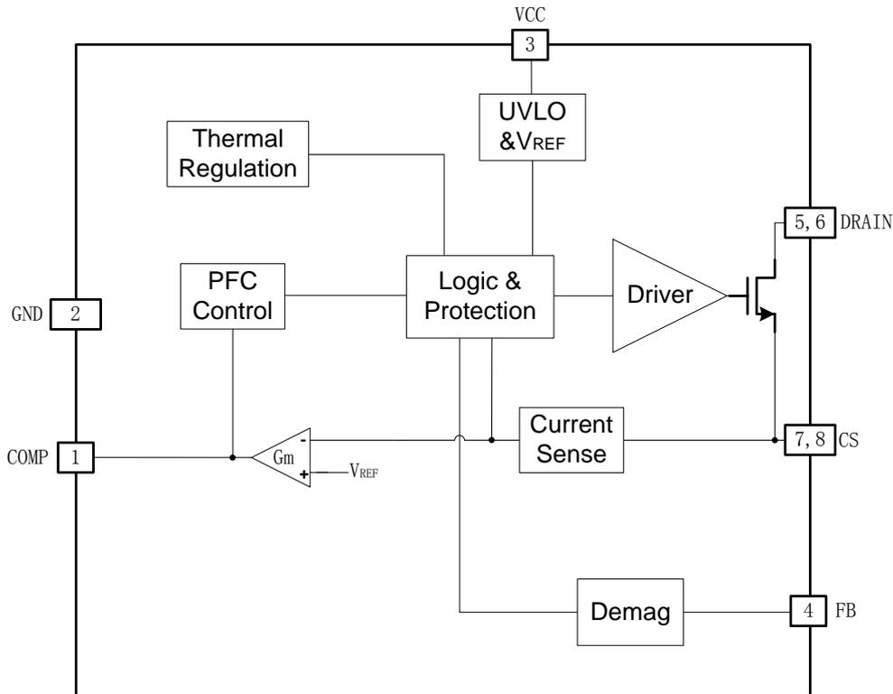
Figure 3. HW9616B Internal Block Diagram
